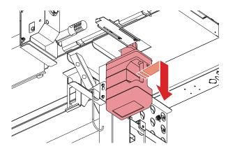
5 Attach the cap to the removed waste ink tank, and use tape to prevent leakage of waste ink.
