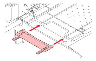
7 Secure the media holder stopper with the screw.
